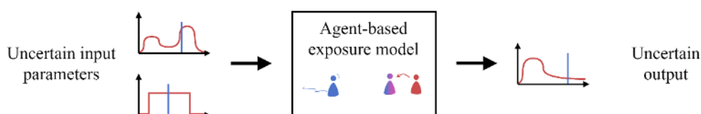
Figure 1: Uncertainties (characterized by probability density functions, red) in the input propagate through the model and yield an uncertain output. Evaluating only one sample (blue) can return a non-representative result.
