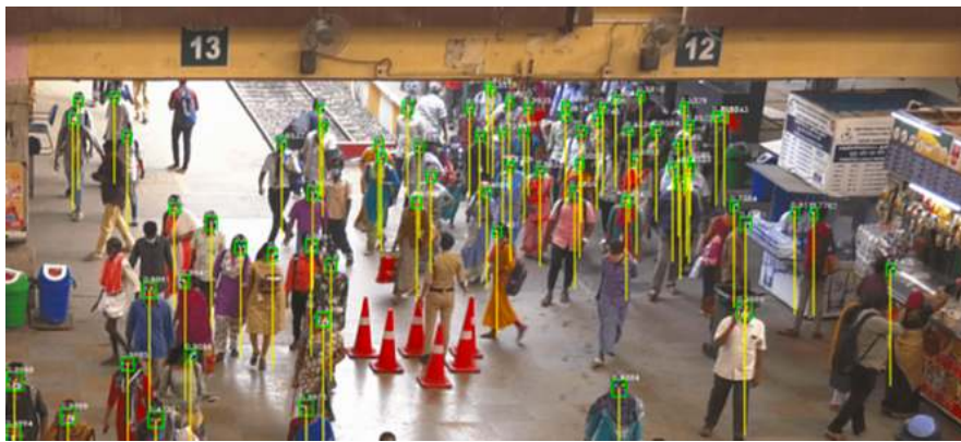
Figure 1: Pedestrians entering the station waiting hall being steered by police officer towards the exit. The deep learning algorithm (RETINA FACE) automatically detects pedestrians (green box), and the yellow line represents pedestrian height.
