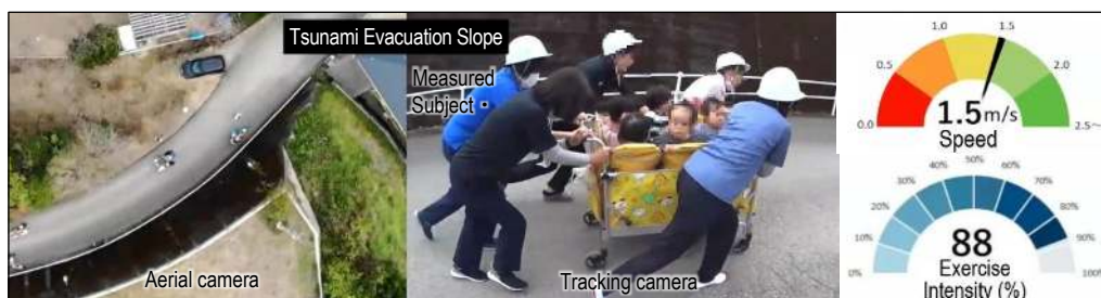
Figure 1: Walking speed and exercise intensity of a nursery worker handling stroller on a steep slope (sample).
